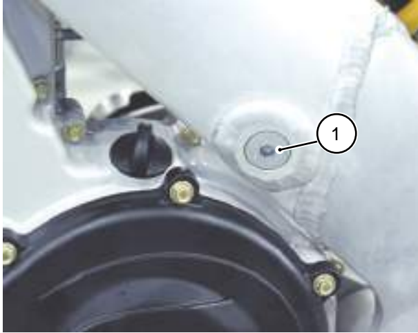
1. Left spar drain bolt
