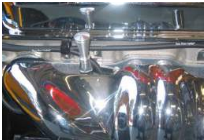
Figure 1.2 Small Block 350 dipstick location.
