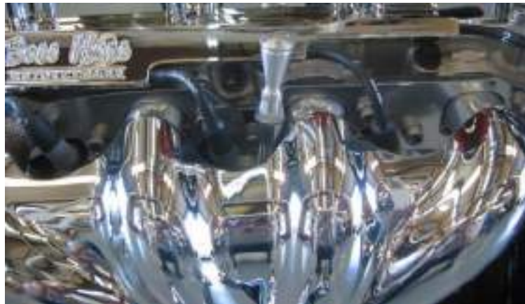
Figure 1.1 Big Block 502 dipstick location.
