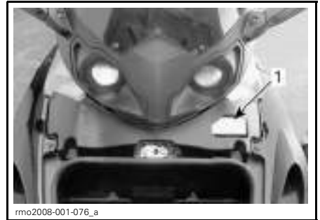
1. Fuse box located under the service cover behind the front storage compartment
