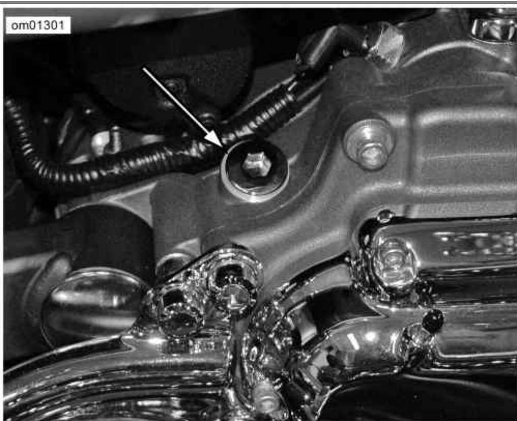
Transmission Filler Plug/Dipstick Location: FXDFSE2
