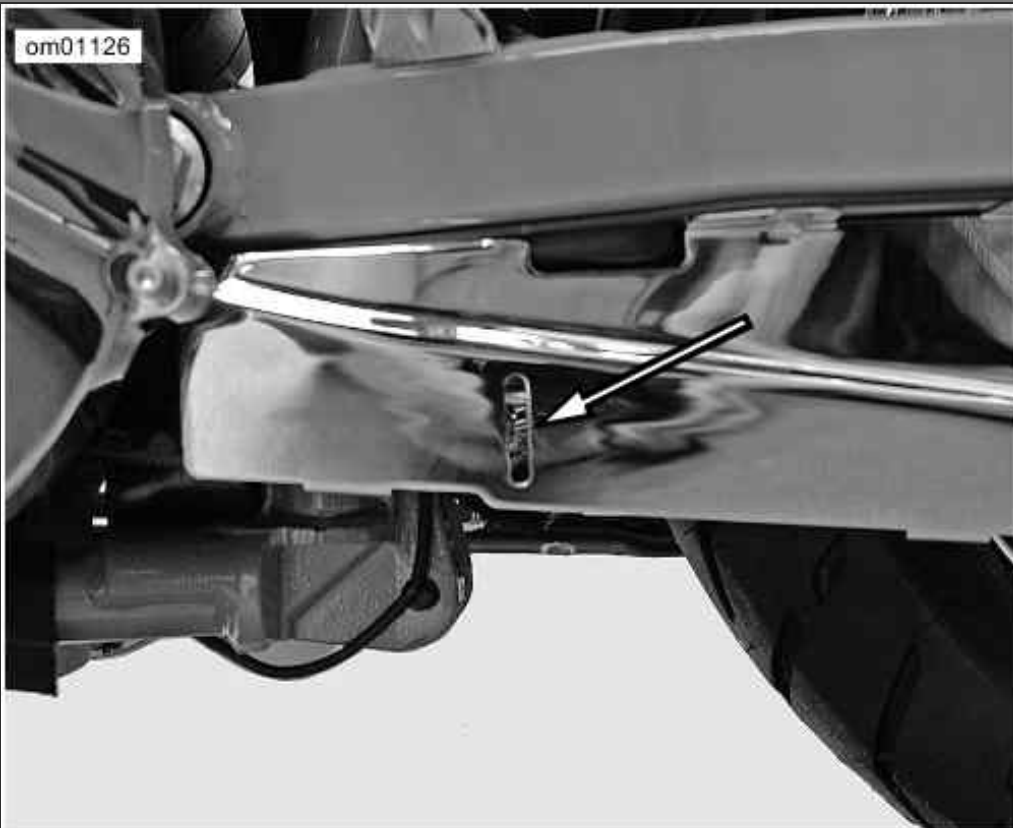
Belt Deflection Window
