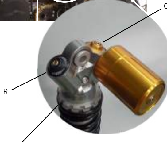
Adjustable rings for the spring pre-charge
