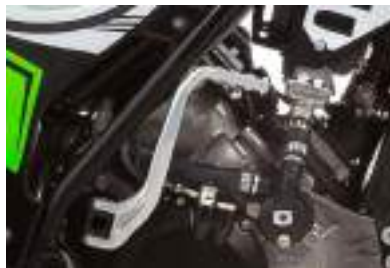
Engine kick-start pedal joints
