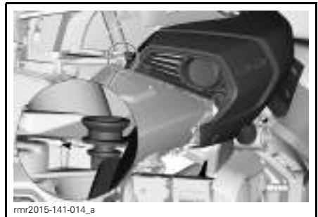
ALIGNING PANELS PROPERLY
