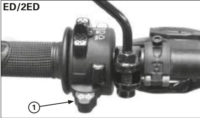
(1) TURN SIGNAL SWITCH
