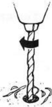
2. Drill hole in stud
