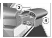
• Insert socket 4 into spacer 3.
