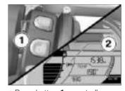
Press button 1 repeatedly until desired heating level 2 is shown.
