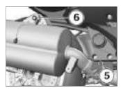
Insert screw 6 and tighten to the specified torque while counter-holding the nut on this inside.
