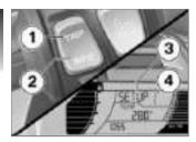
SETUP **3** has been started. The separating line **4** is hidden.
