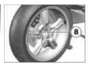
• Fit five screws **8** and tighten diagonally with specified torque.
