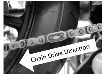
Master link clip orientation
