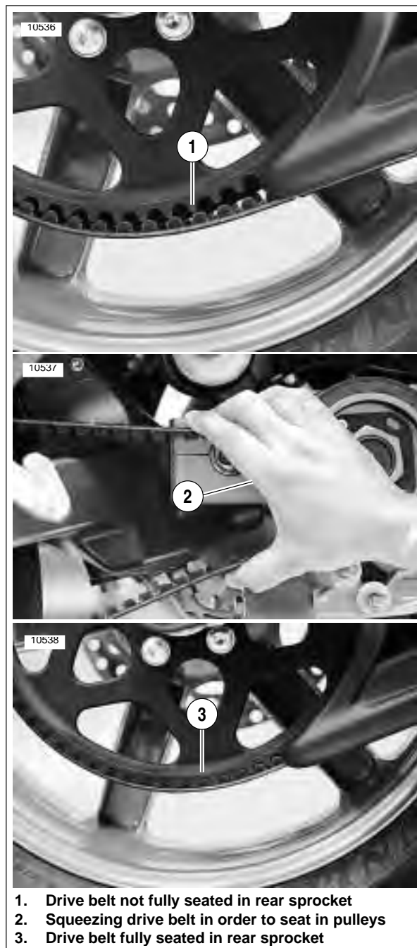
Figure 6-42. Seating Drive Belt Into Pulley Teeth
