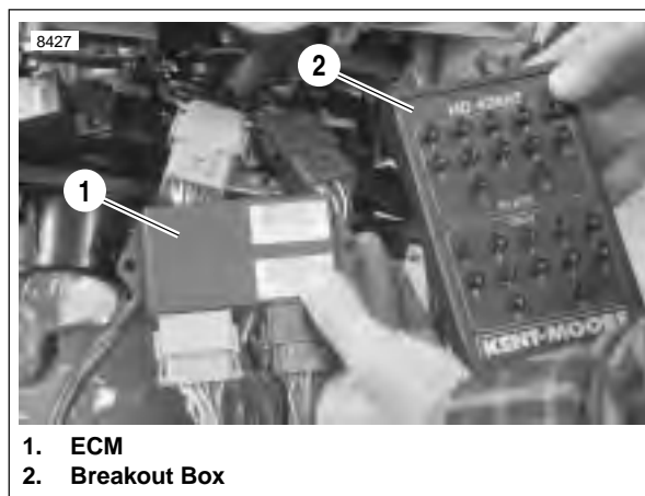
Figure 4-10. Installed Breakout Box
