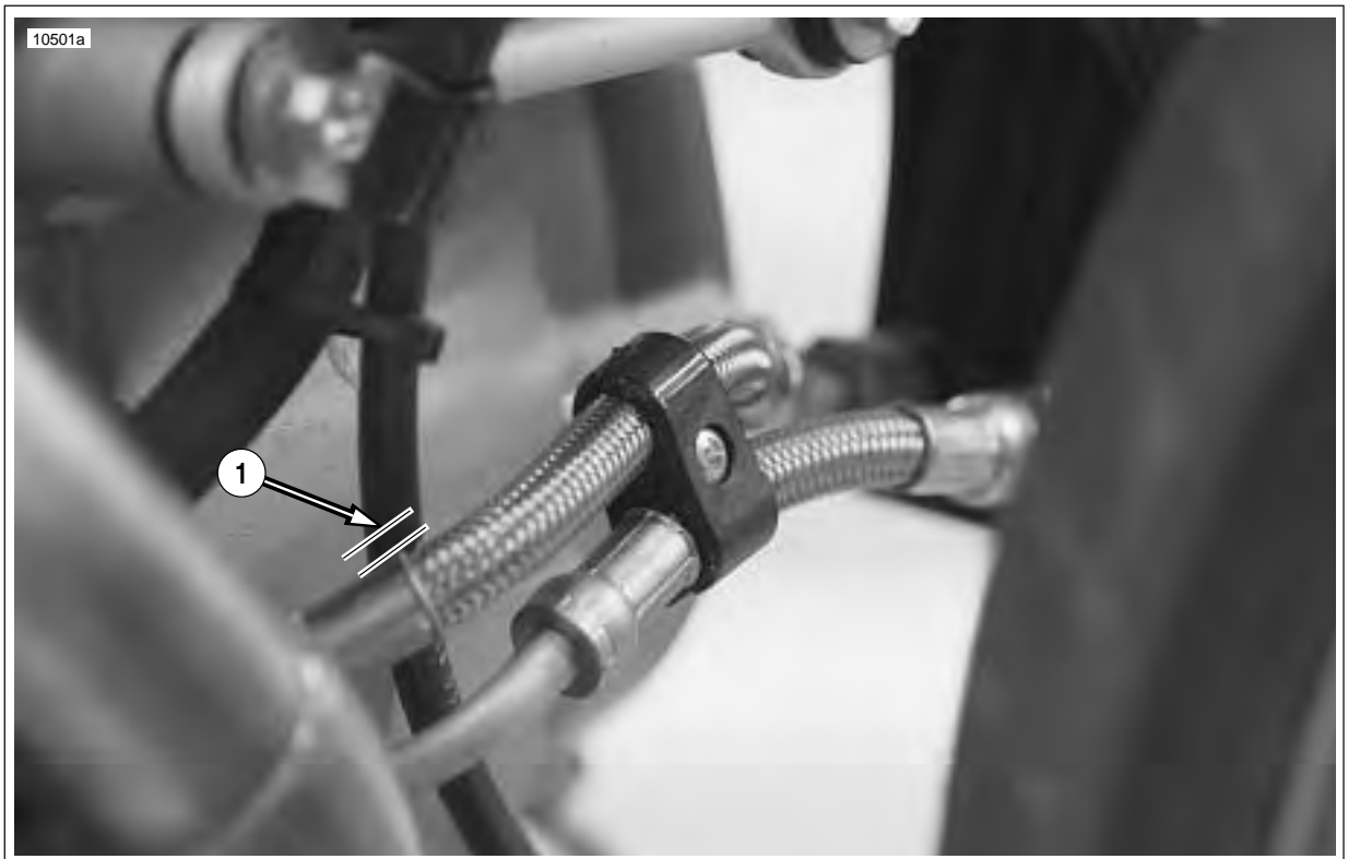
Figure 3-10. Oil Cooler Feed and Return Oil Line 1/8-1/4 in. (3.175-6.35 mm) Clearance to Clutch Cable
