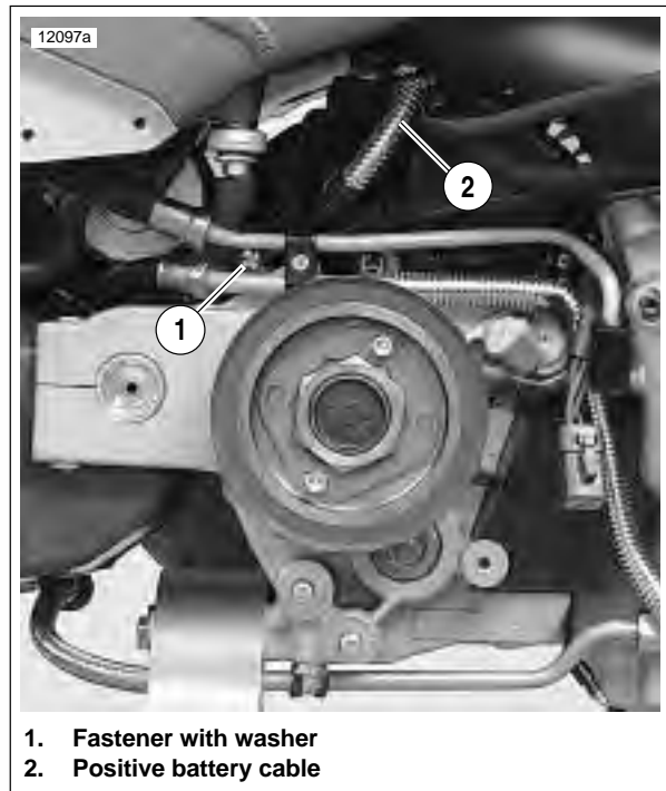
Figure 7-40. Positive Battery Cable (Protective Boot Not Shown)
