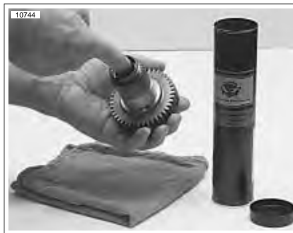
Figure 6-76. Lubricating Main Drive Gear Needle Bearings
