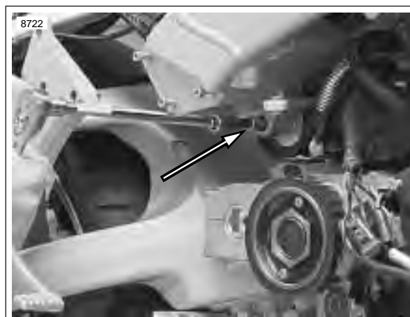
Figure 3-41. Installing Rear Isolator Bolt (Typical)
