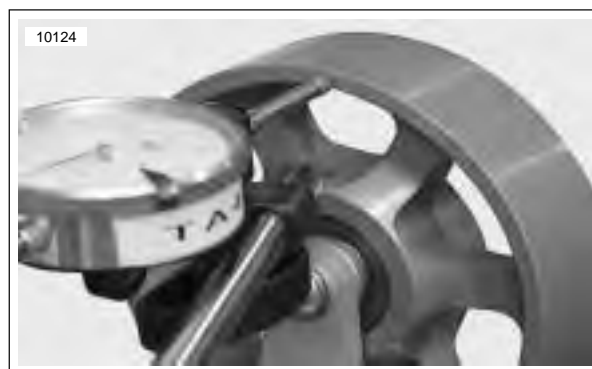
Figure 1-26. Checking Lateral Sideplay on Idler Pulley with a Dial Indicator
