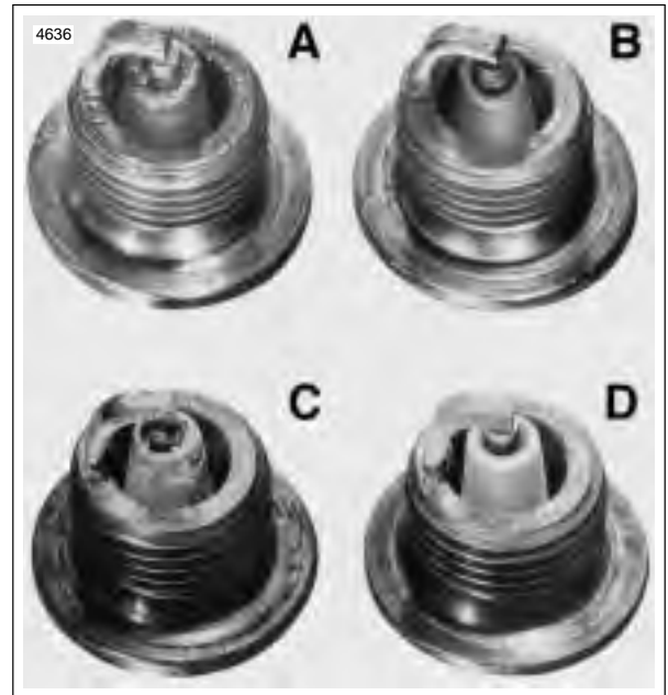
Figure 1-37. Typical Spark Plug Deposits
