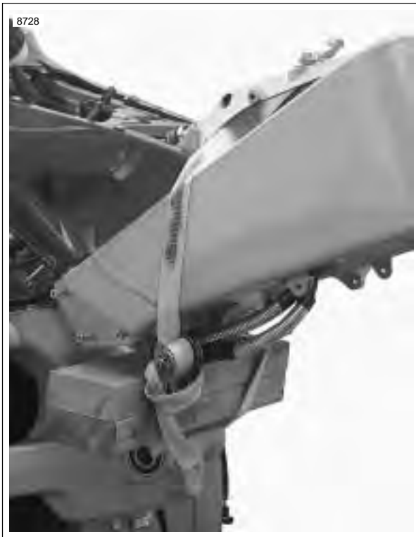
Figure 3-31. Securing Vehicle for Relocation (Typical)
