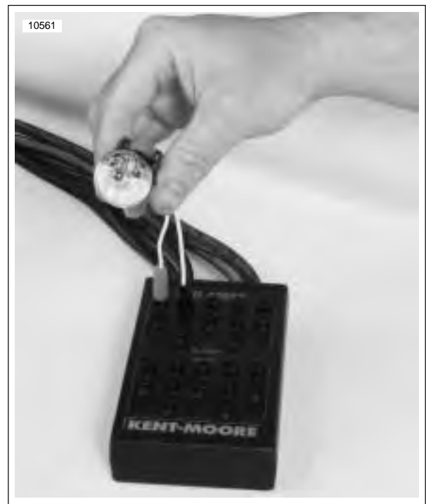
Figure 4-50. Testing Ignition Coil Connectors
