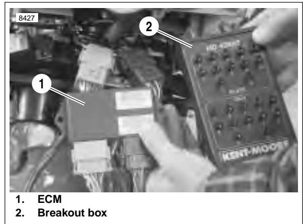
Figure 4-54. Installed Breakout Box
