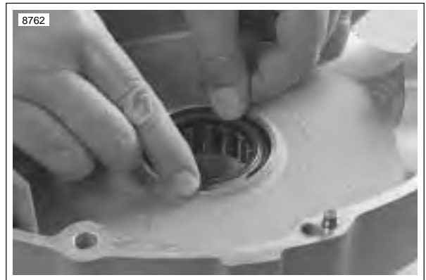
Figure 3-140. Removing Sprocket Shaft Bearing Retaining Ring
