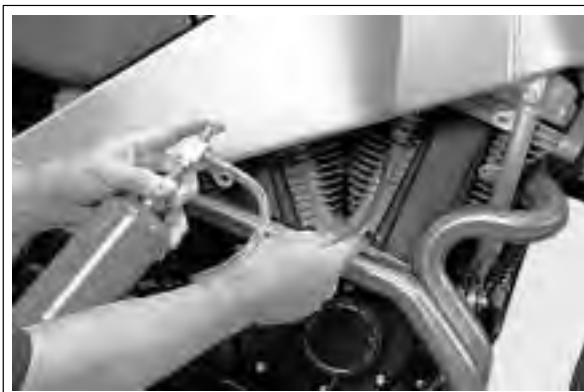
Figure 4-112. Checking for Intake Leak
