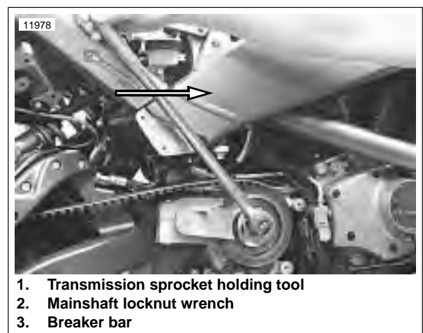
Figure 6-102. Removing Transmission Sprocket Locknut
