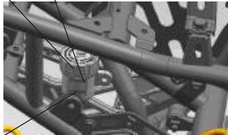
① Rear brake fluid reservoir ② Upper level line ③ Lower level line
