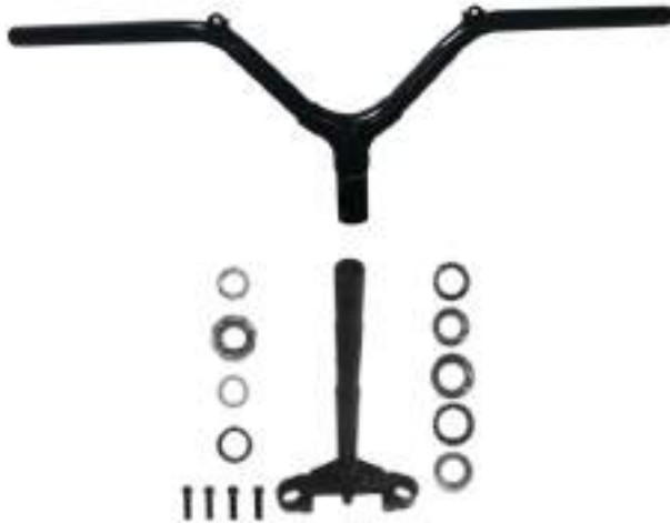
Structure of direction column and direction handle
