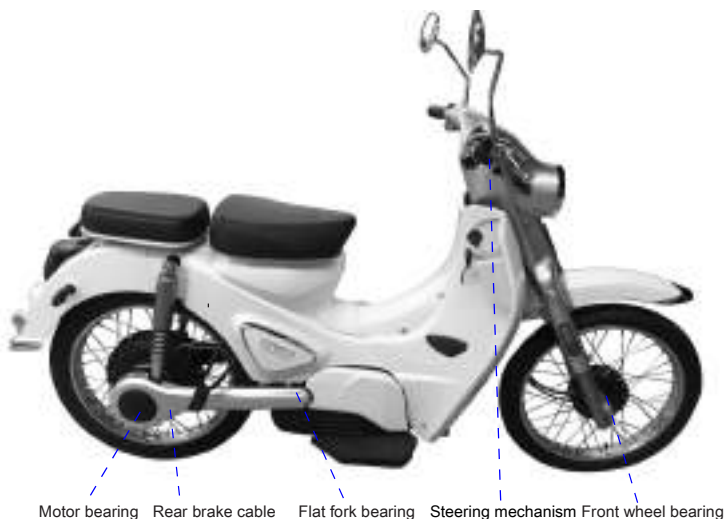
Lubrication parts of ZS1500D-6 electric vehicle
