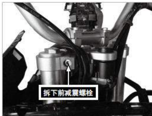
Remove the front shock absorbing bolt
