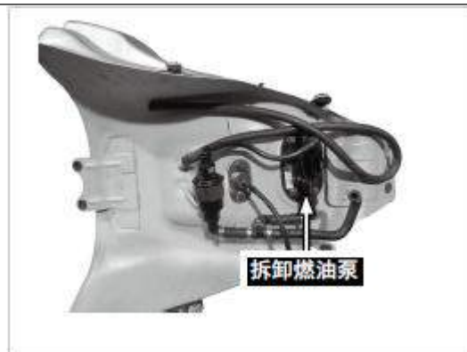
Removing fuel pump
