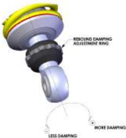
11. Adjustment of rebound damping
