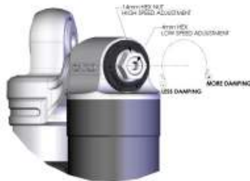
12. Adjustment of compression damping
