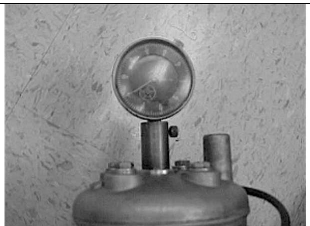
Figure 36, Using a dial indicator to measure piston height for setting ignition timing.
