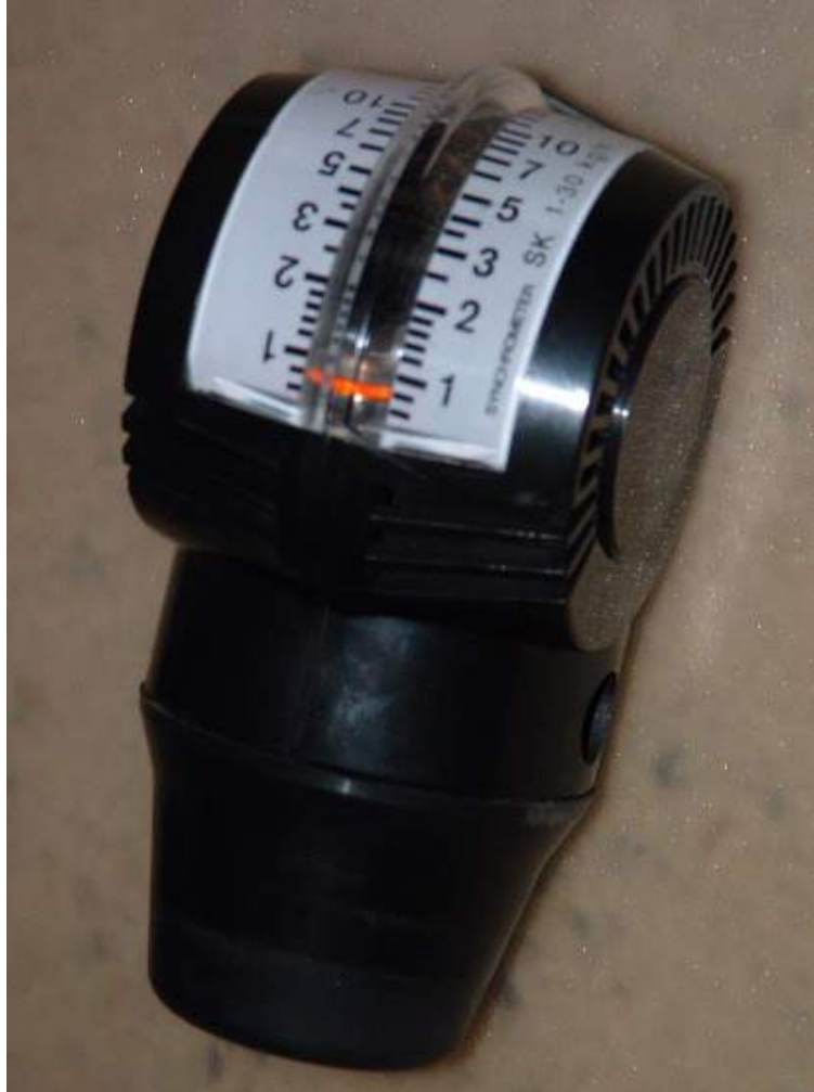
Appendix 2 Synchrometer (an alternative to tuning) Used this on my 912 and it works great
