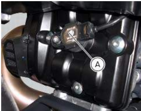
Installation location of horizontal cylinder coil (A).
