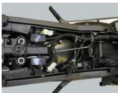
To access the tail light - turn indicators unit, remove the seat as described in Sect. 5 - 3, " Removal of the seat " and the tool tray cover as described in Sect. 7-17, " Removal of the tool tray ".
