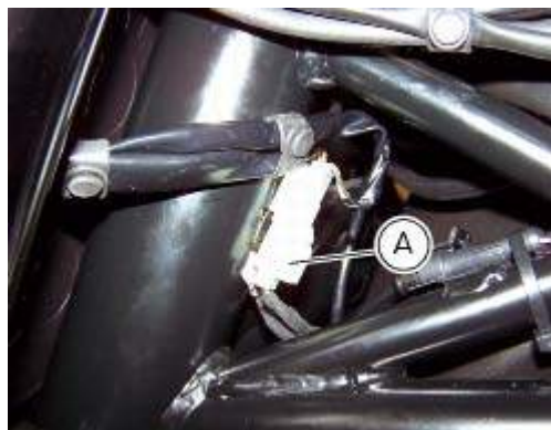
(A) low / high beam and parking light connections Rear running light and stop light connection.
