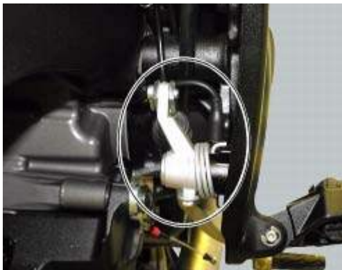
Rear brake button mounted near lever operating brake pump. The button is normally closed (when the brake lever does not press on the button because it has been pressed by enough to cause a braking effect, the contacts close, short circuiting the contacts).
