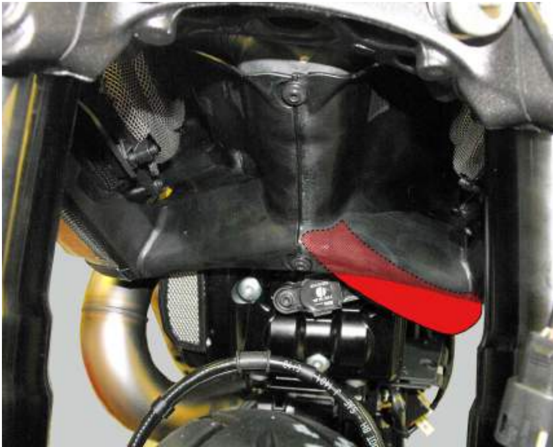
Cooling system: coolant expansion tank
