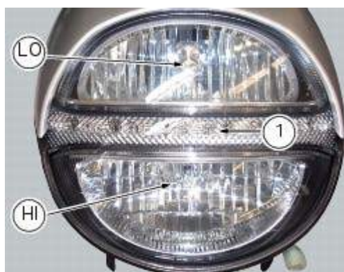
The figure shows the locations of the low beam bulbs (LO), high beam bulbs (HI) and the parking light LED light unit (1).
