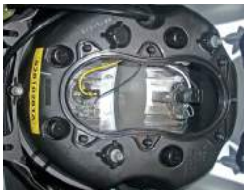
Rear view of the headlight showing the high and low beam light connections and the connection for the LED power module at the centre, with the connector cable.
