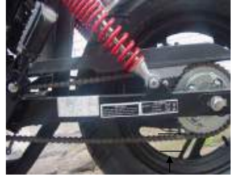
Chain tolerance: 15-25mm
