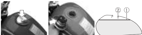
①Fuel level ②Fuel tank
