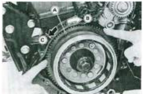
A. Starter Clutch Gear C. Locked. B. Turns freely.
