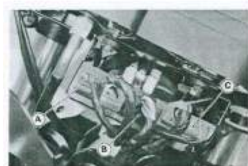
A. Engine Stop Switch 6-pin Connector (Red) B. Ignition Switch 6-pin Connector (Black) C. Starter Lockout Switch 3-pin Connector
