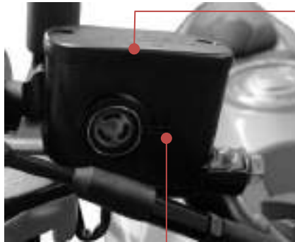
Front brake fluid storage tank
