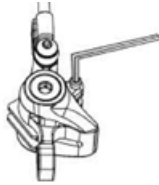
Unscrew the retainer bolt should be 3-5 Nm.
