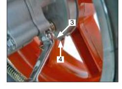
Adjusting the rear wheel brake
