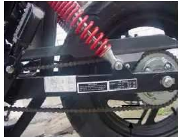
Chain tolerance: 15-25mm
