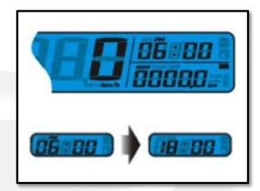
**STOPWATCH:** Press the **Select button** during main screen to switch from Clock to Stopwatch.
