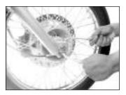
• Remove the axle nut along with washer.
