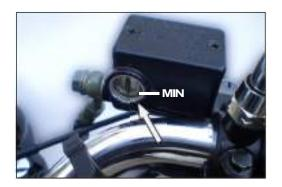
9. Lub oil level should be in between "MAX " & "MIN" Level. Top up if necessary. Do not overfill above maximum level.
