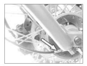
• Tighten the pinch bolt on the RH fork guide.
