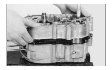
Remove the gasket and dowel pins.
