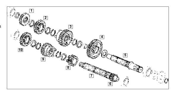
Assemble the shift drum, countershaft and mainshaft assemblies.
