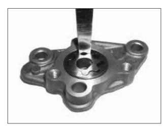
Measure the pump body clearance.
