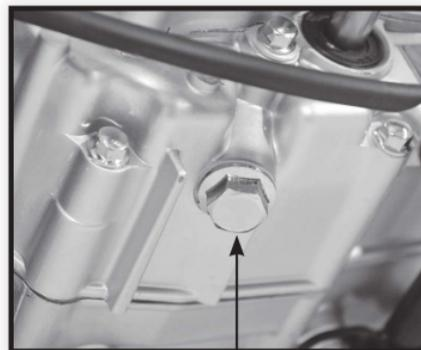
**PARAFUSO DE DRENAGEM****5.4. VELA DE IGNIÇÃO**
