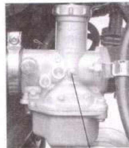
Idling speed adjusting screw
