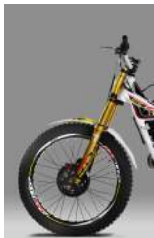
b) On the left-hand side of the suspension you can set the length.
