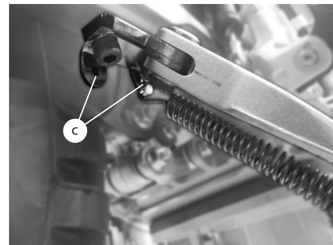
c) Adjustment holes in the side stand
