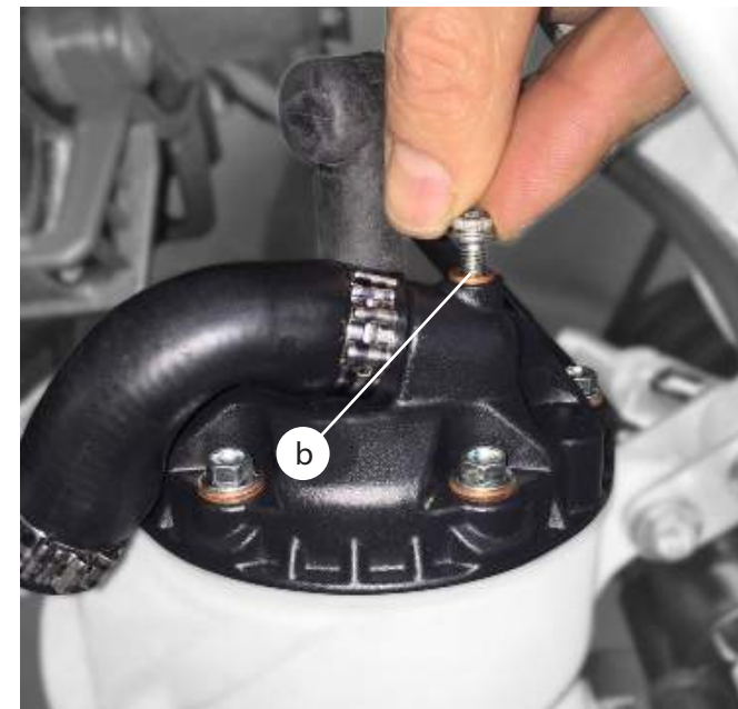
b) Bleed screw for the coolant, located in the cylinder head.
