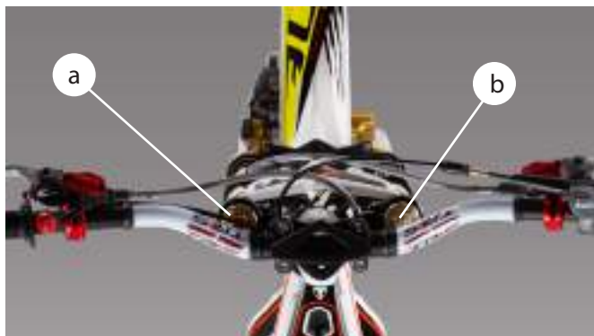
a) Spring preload; b) Adjusting the length
