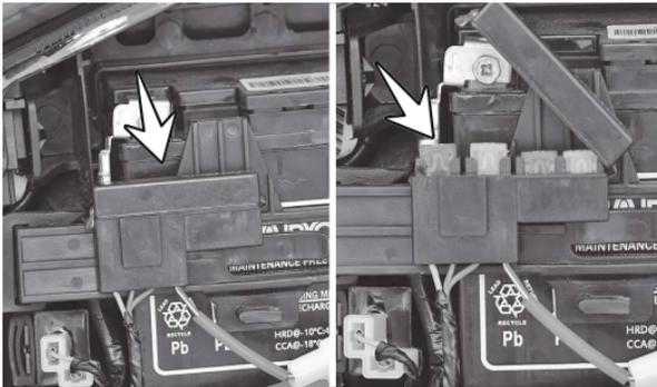
4. Replace the fuse with a new (extra fuses are provided inside the fuse case itself).
