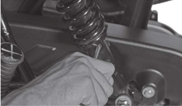
Adjust the spring pre-load by shifting the adjuster to the required notch according to the different load conditions. The more you compress the spring, the suspension becomes more stiff.
