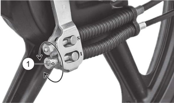
3. Turn the adjuster nut at bottom side (1) in the slot marked as "I" in clockwise direction for reducing the free play or in anti-clock wise direction for increasing the free play.
