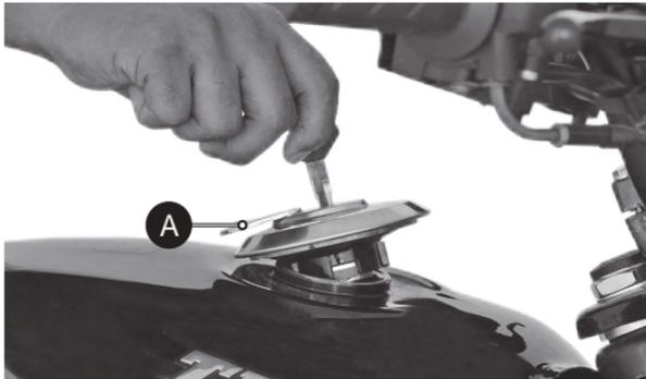
To open the fuel tank cap, move away the protection lid (A) from its position. Insert the key into the lock and turn it in clockwise. The tank cap ejects automatically. Take out the cap along with the key.
