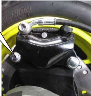
Image 45 Disassemble the bolts
