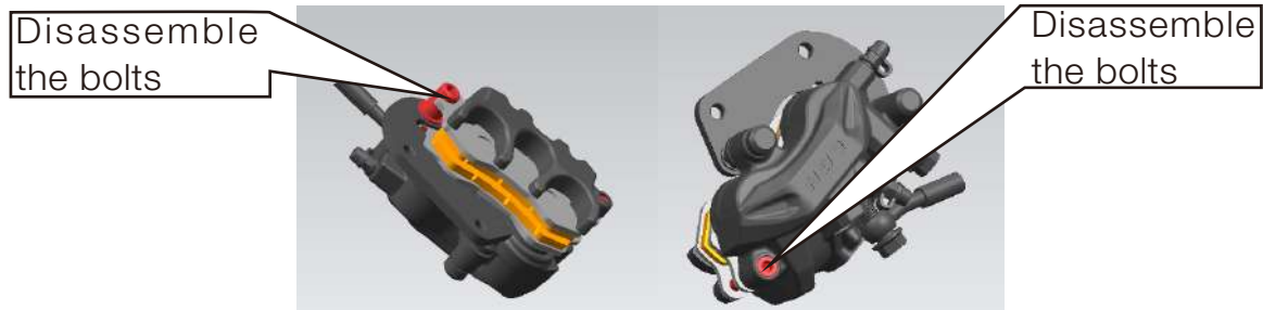
Image 42 Disassemble the bolts
