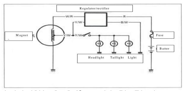
On the other hand, lighting coil supplies AC current to the headlight, taillight, and meter light under the regulated condition.
