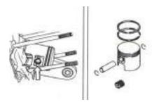
Remove the piston pin and piston.
