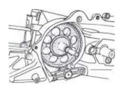
Remove the clutch housing with the special tool.
