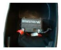
Measure the voltage between the +ve and –ve terminal of Battery charge the Battery if the voltage is below the specified limit.
