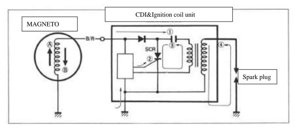
The ignition system consists of a flywheel magneto, a CDI&Ignition coil unit and a spark plug. 1 As the rotor generates, an AC current is induced in the coil. Then current induced in the A direction charges up the capacitor.
