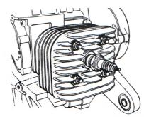
If cylinder head nuts are not tightened to the specified torque, may result in leakage of compressed fuel-air mixture and reduce output, tighten the cylinder head nuts in the following procedures:
