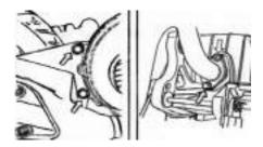
Remove magneto rotor nut.
