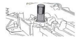
Crankcase bushing disassembly
