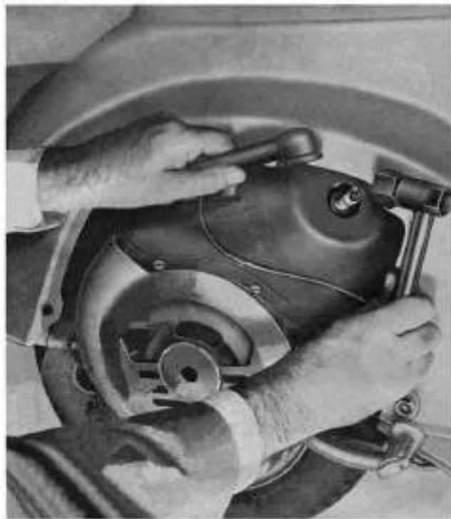
Fig. 10 - Dismantling spark - plug
