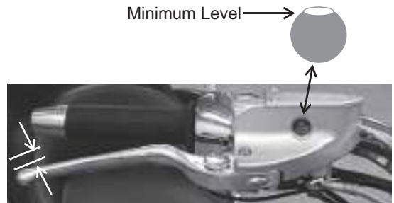
Resistance at 3/4 inch (19 mm)
