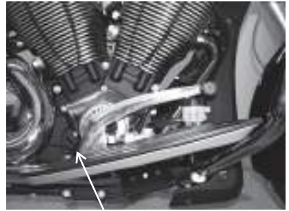
Oil Fill Cap/Dipstick
