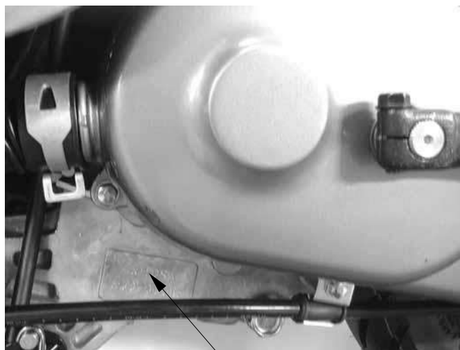
Location of Engine Serial Number
