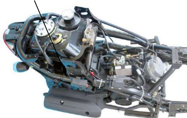
A.C. Generator Wire Connector
