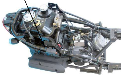
A.C. Generator Wire Connector
