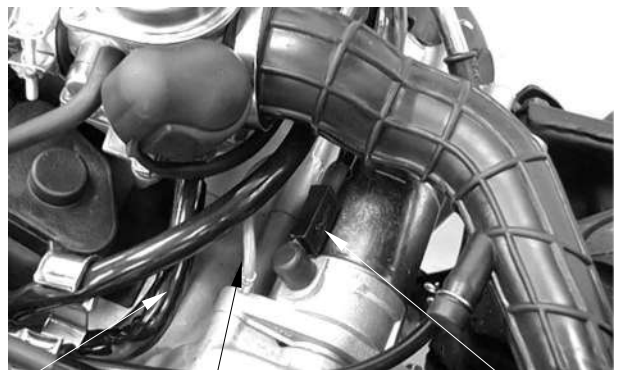
fuel tube Earthr Cable Starter Motor Cable
