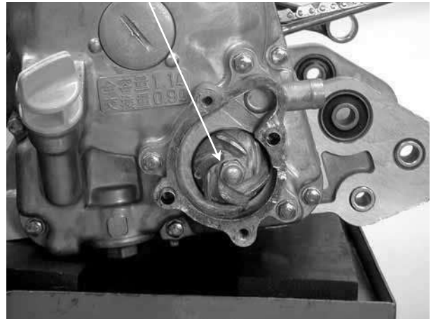
Impeller (Left Hand Threads)
