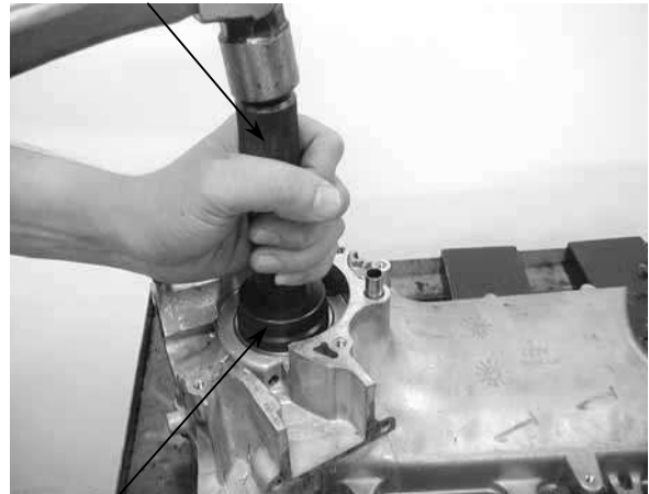
Bearing Outer Driver, 42x47mm Pilot, 20mm
