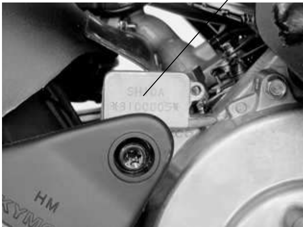
Location of Engine Serial Number
