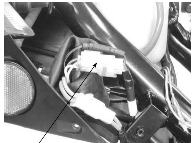
A.C. Generator Connector
