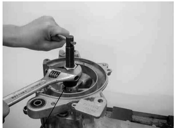
Crankcase Assembly Tool
