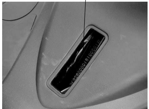
Location of Frame Serial Number
