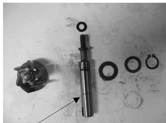
Water pump shaft
