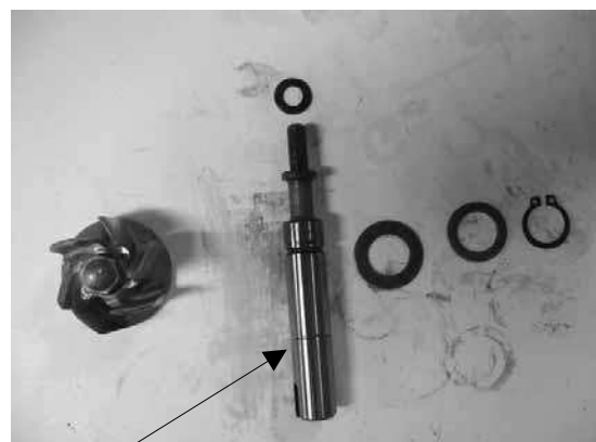
Water pump shaft
