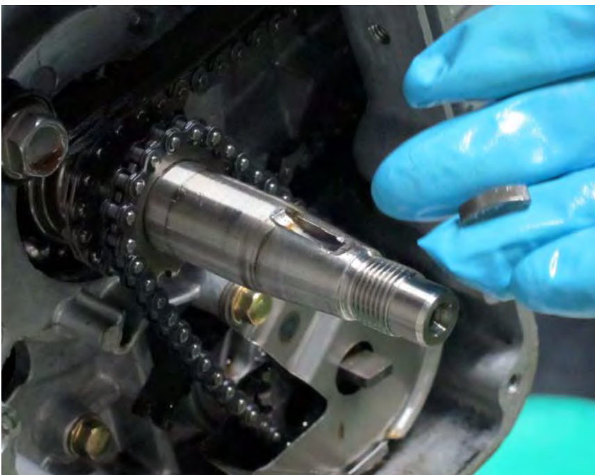
Remove the woodruff key from the crankshaft.
