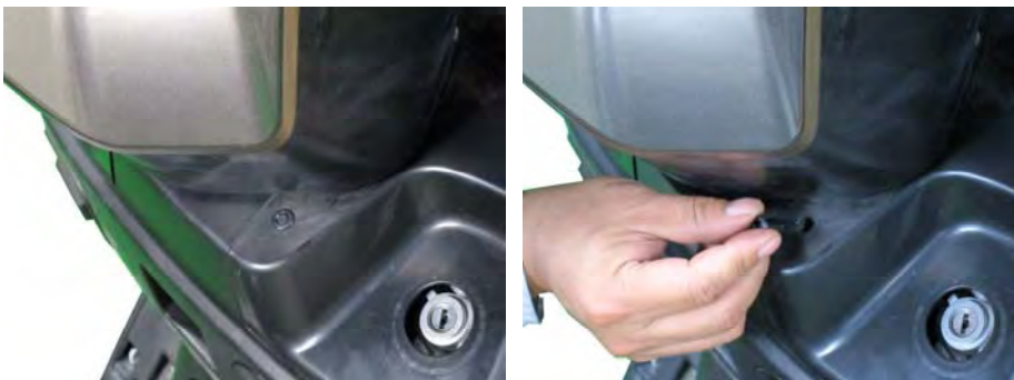
Remove the two push pins below the handlebar. Depress the head of the fastener center piece. Pull out the fastener.
