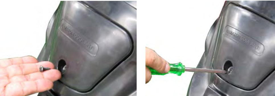
Install the radiator coolant panel screws and tighten securely with a #2 Phillips screwdriver.
