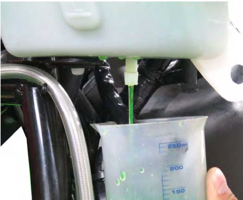
Pull back the clamp and free the overflow hose from the bottom of the reserve tank. Allow the coolant in the reserve tank to drain into the container.
