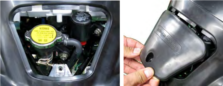
Install the radiator cap access panel.
