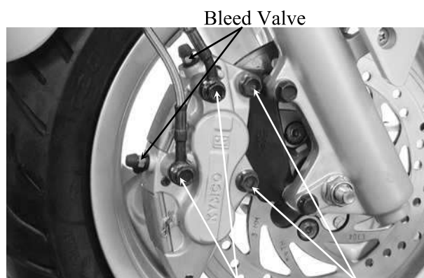
Bleed Valve Fluid Tube Bolt Bolts
