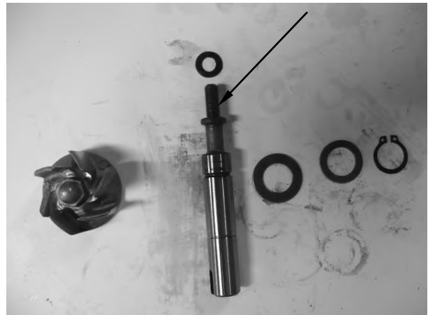
Water Pump Shaft
