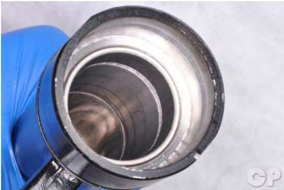
Inspect the slider bushing and replace it as needed.
