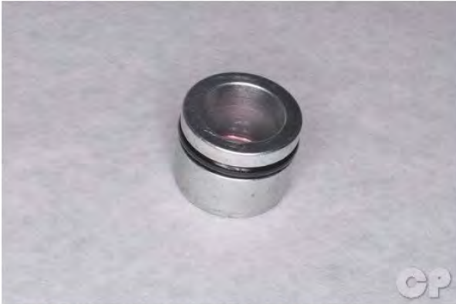
Inspect the top plug O-ring O-ring and replace it if needed.
