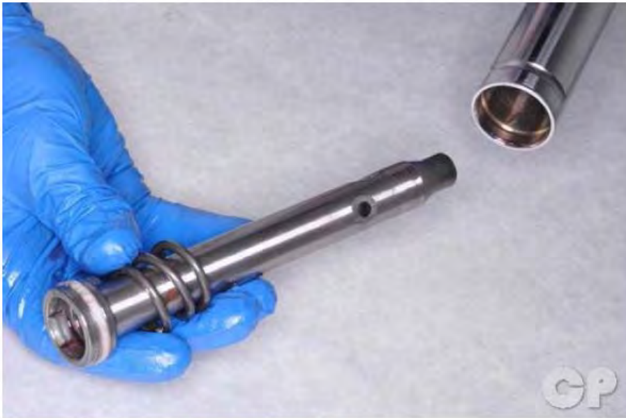
Remove the damper rod and rebound spring.
