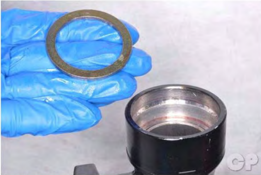
Place the spacer into the fork slider.
