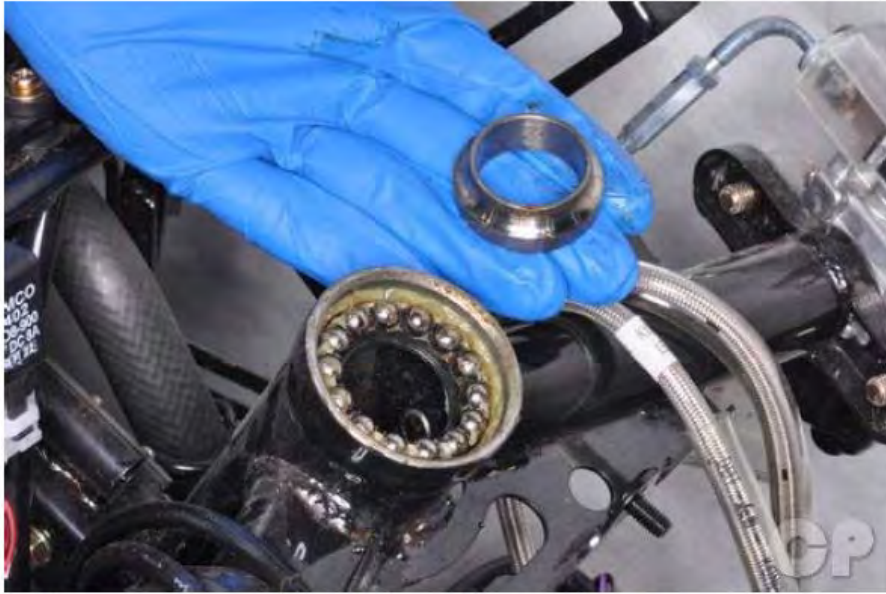
Set the upper bearing inner race into the upper bearing.
