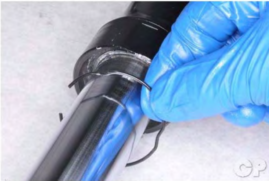
Insert the stopper ring into its groove.
