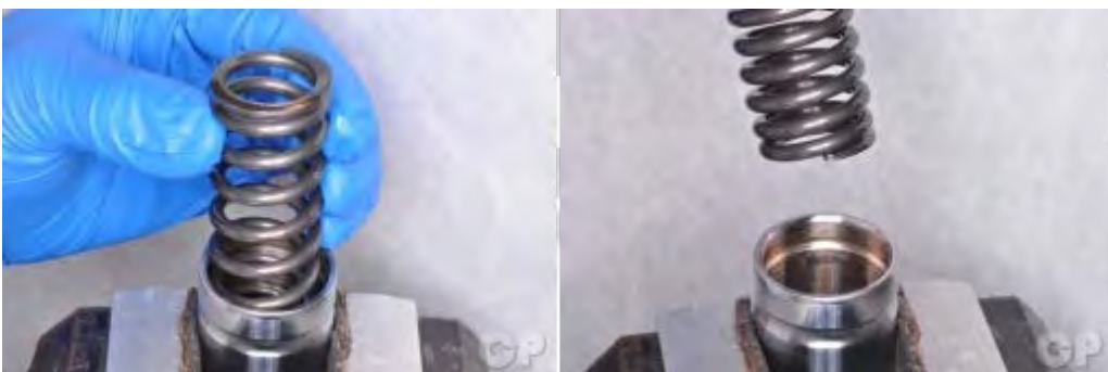
Lift out the fork spring.
