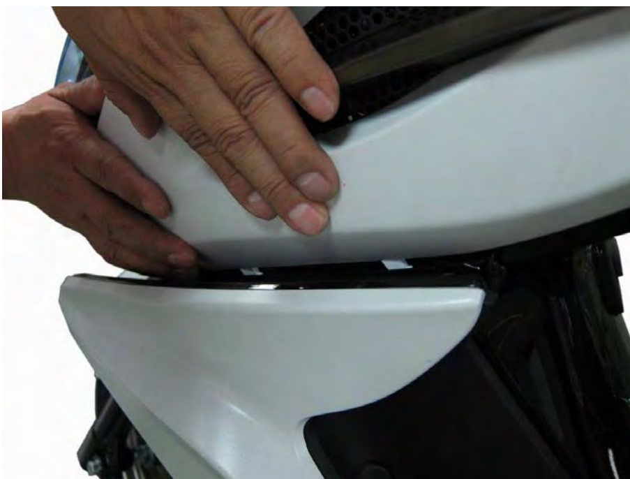
Carefully Align the side molding and side skirt with hand on each side.
