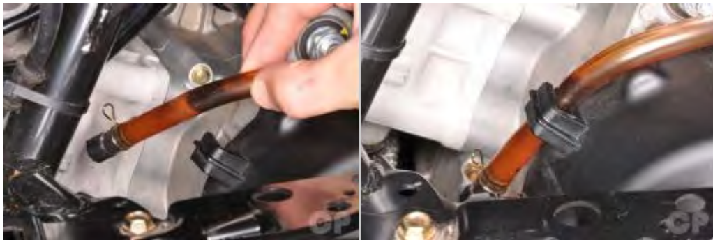
Connect the transmission vent hose.
