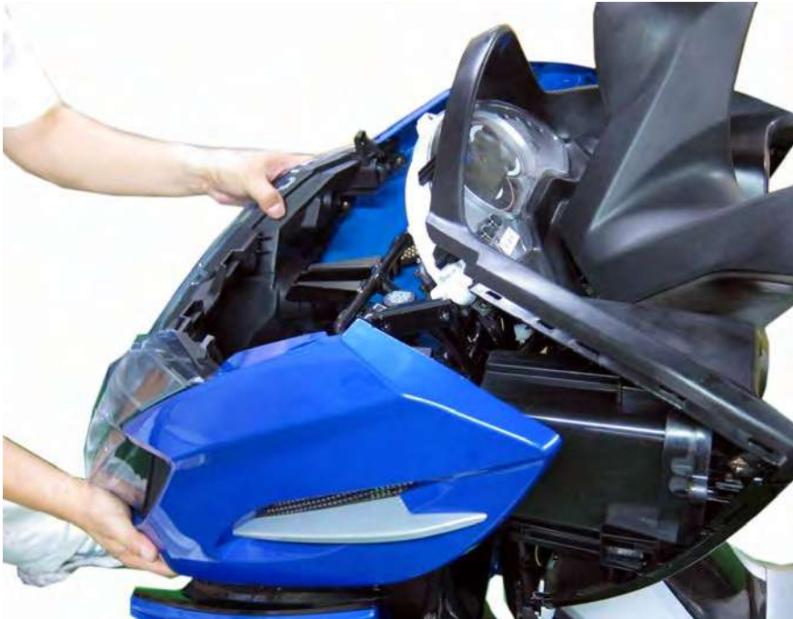
Align front cover tabs. Install the front cover.
