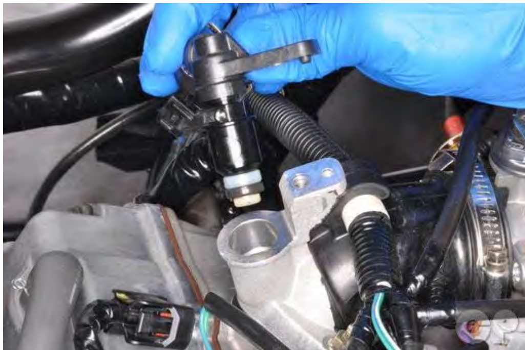
Lift the fuel injector out of the intake pipe.
