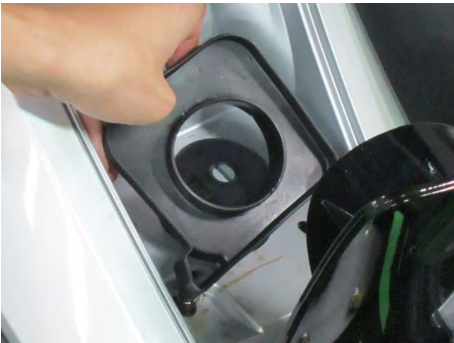
Remove the Lid fuel cap maint.
