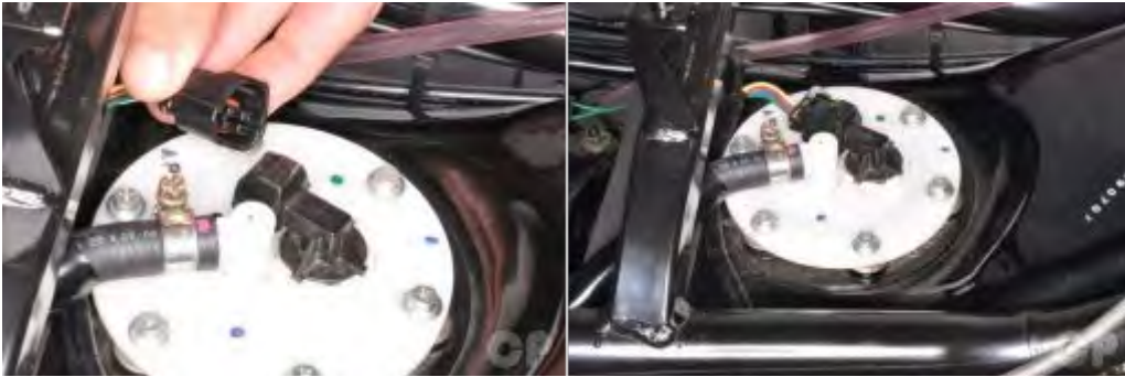
Plug in the fuel pump connector.
