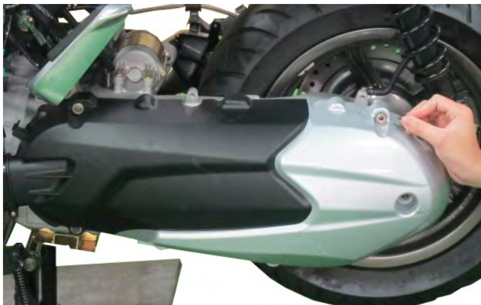
Install the belt case plastic cover.
