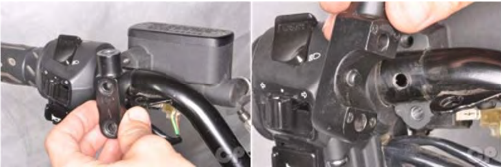
Remove the master cylinder clamp.
