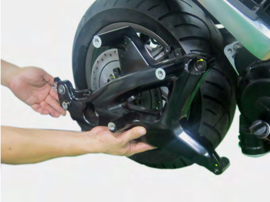
Fit the rear fork into place.
