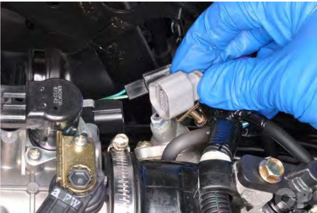
Unplug the throttle position sensor (TPS) connector.
