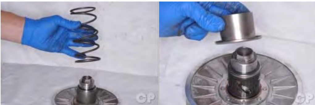
Remove the collars and spring.
