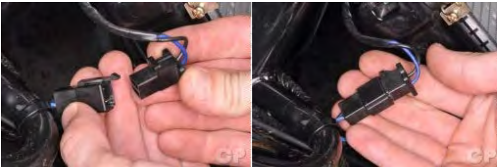
Plug in the cooling fan motor connector.
