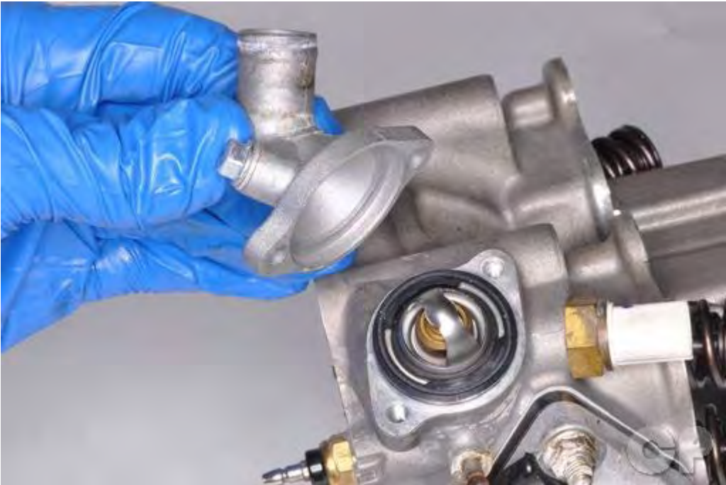
Lift off the thermostat cover.
