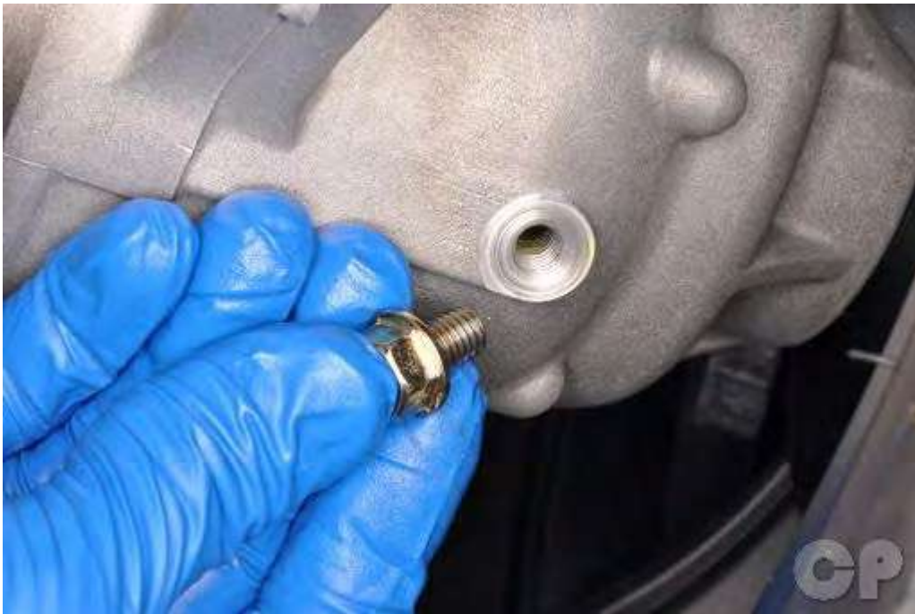
Thread in the final drive oil level check bolt.
