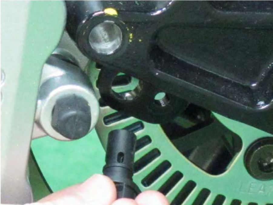
Remove the front wheel speed sensor from the bottom of the right fork leg.
