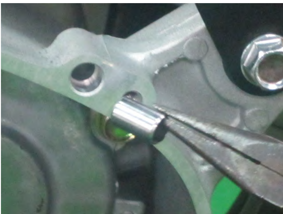
Remove the two dowel pins.
