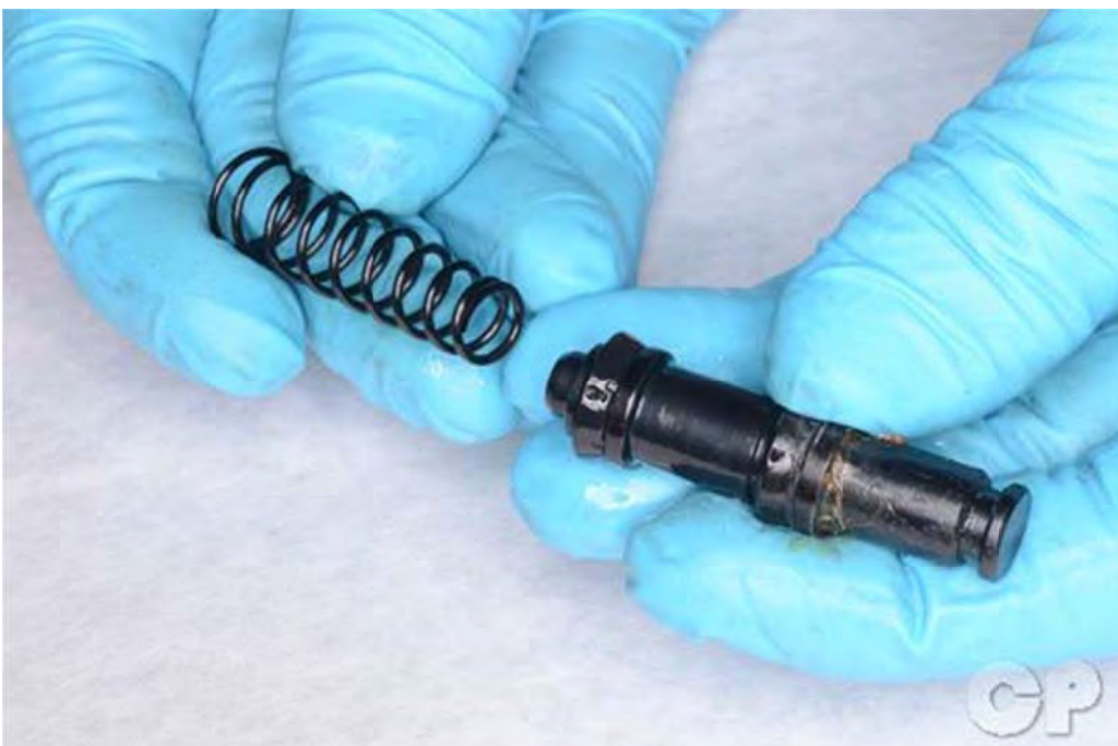
Remove the spring from the piston and
