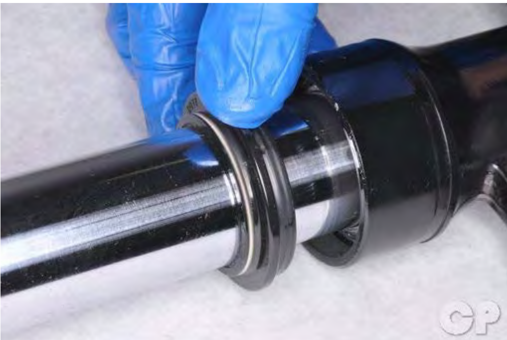
Install the dust seal securely into the outer fork tube.
