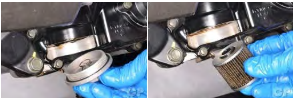
Remove the oil filter cap with spring and take out the used oil filter.
