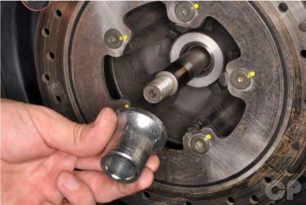
Slide on the rear axle collar.
