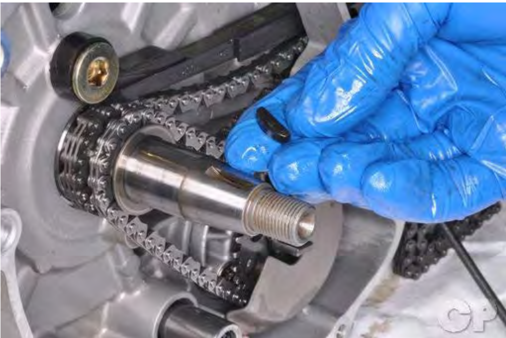
Remove the woodruff key from the crankshaft.
