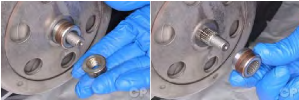
Remove the driven pulley nut and bushing.
