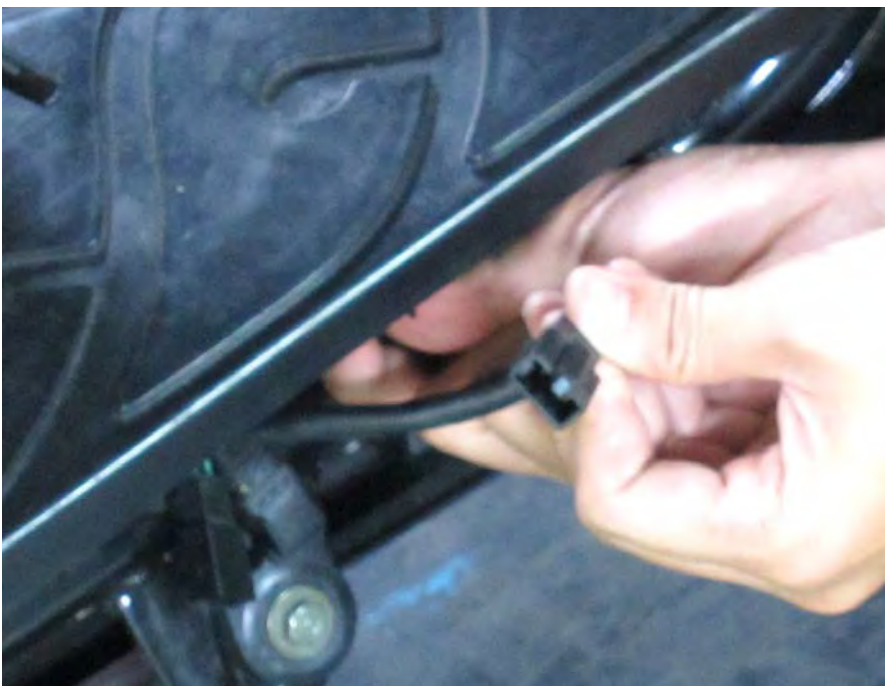
Plug in the side stand switch connector.
