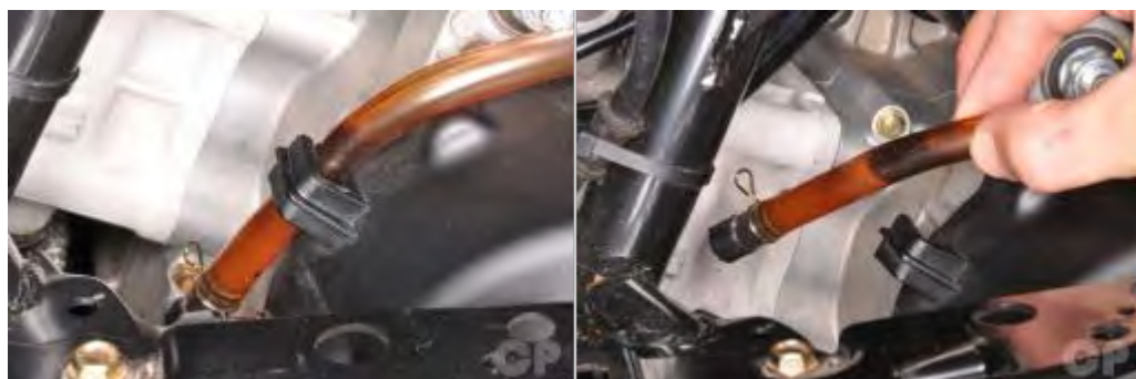
Disconnect the transmission vent hose.
