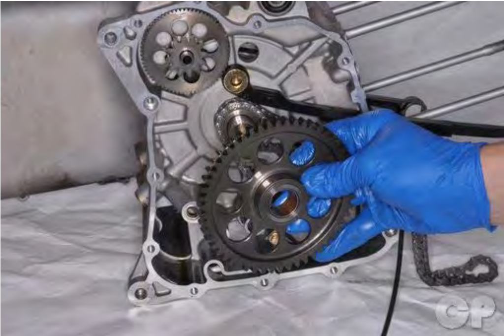
Slide the starter driven gear off of the crankshaft.
