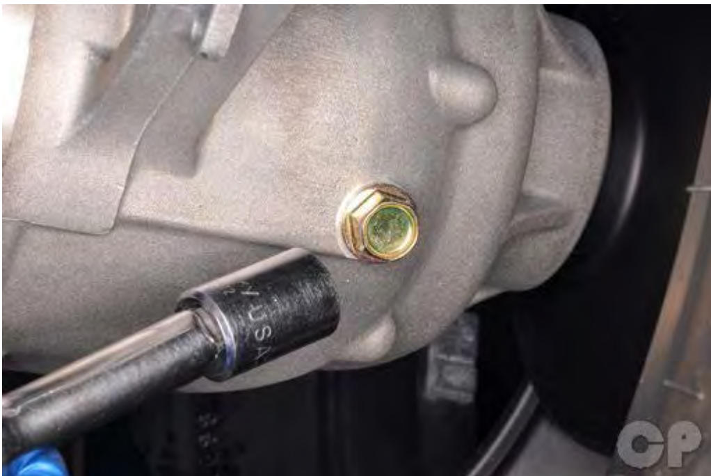
Install the oil check plug and torque it to specification with a 12 mm socket.
