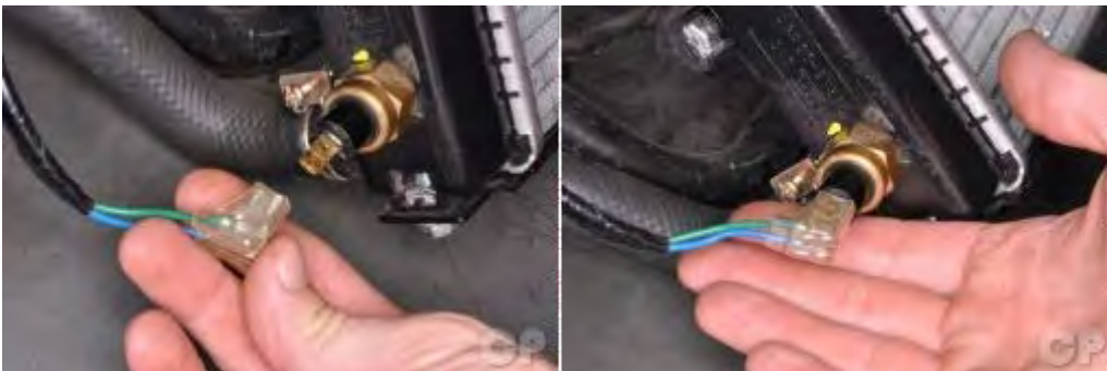
Plug in the thermostatic switch connectors.
