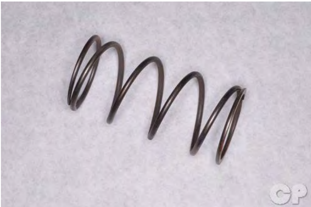
Measure the free length of the clutch spring. Replace the spring if the measurement fails to meet the service limit.
