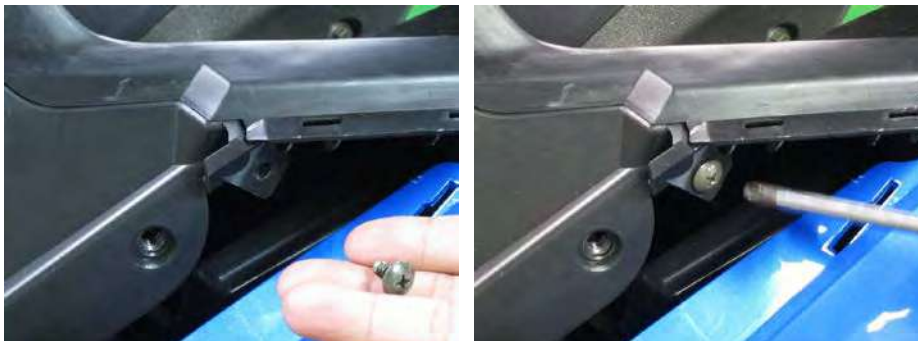
Install the two screws mounting on the front cover meter on each side.
