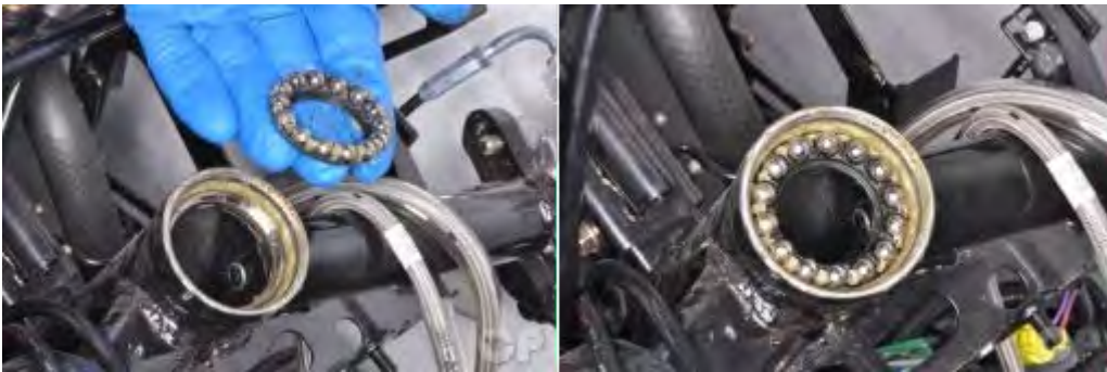
Lubricate the upper bearing with grease and set it into place.
