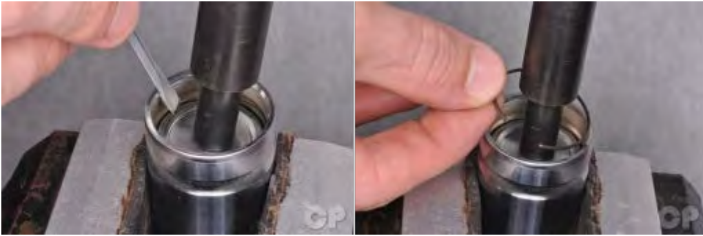
Push down on the top plug and remove the snap ring.
