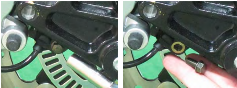
Remove the speedometer sensor mounting bolt with an 8 mm socket.
