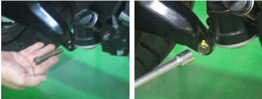
Install the two rear fork mounting bolts and tighten them securely with a 14 mm socket.
