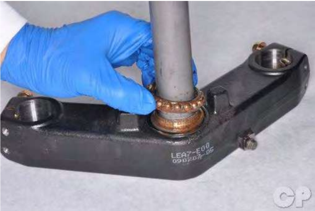
Lubricate the new lower bearing with grease and place it on the steering stem.
