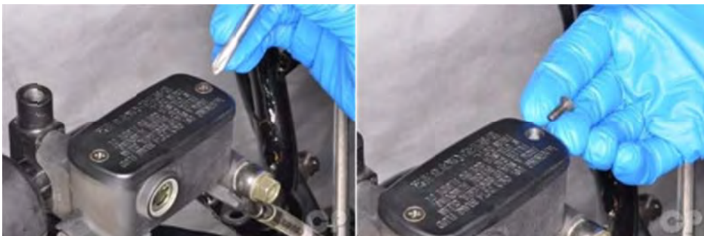
Remove the two master cylinder cover screws with a #2 Phillips head screwdriver.
