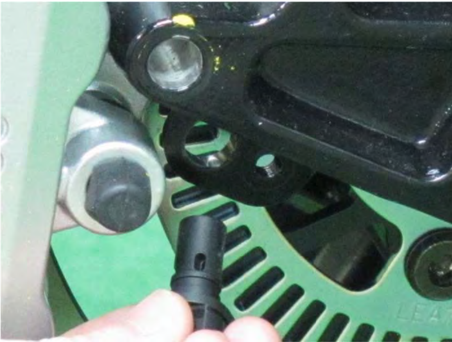
Remove the speedometer sensor.
