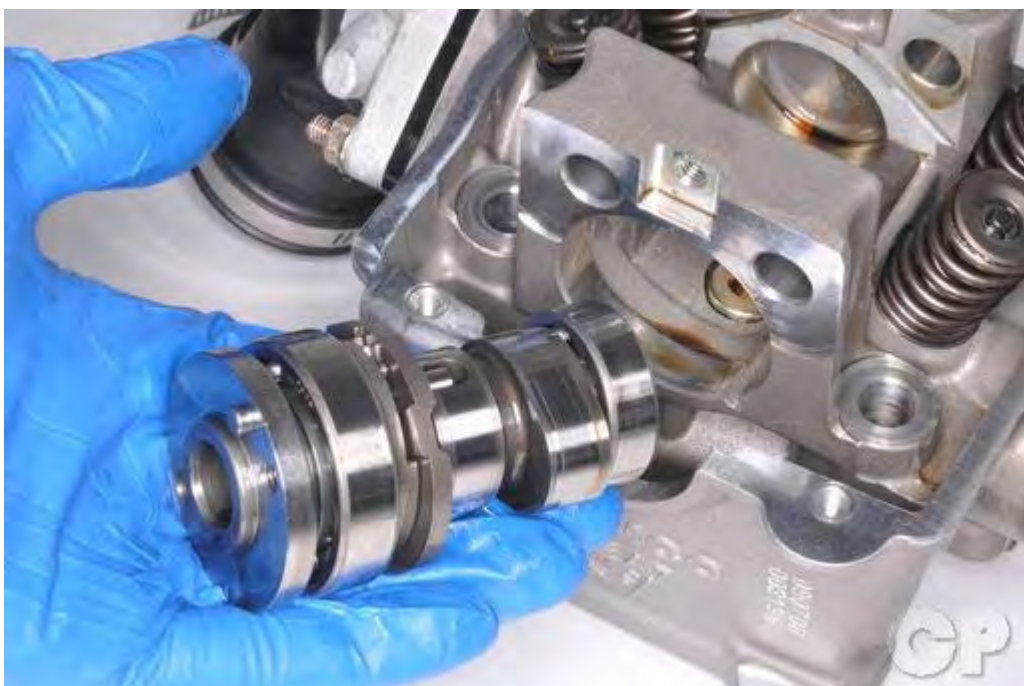
Remove the camshaft from the cylinder head.
