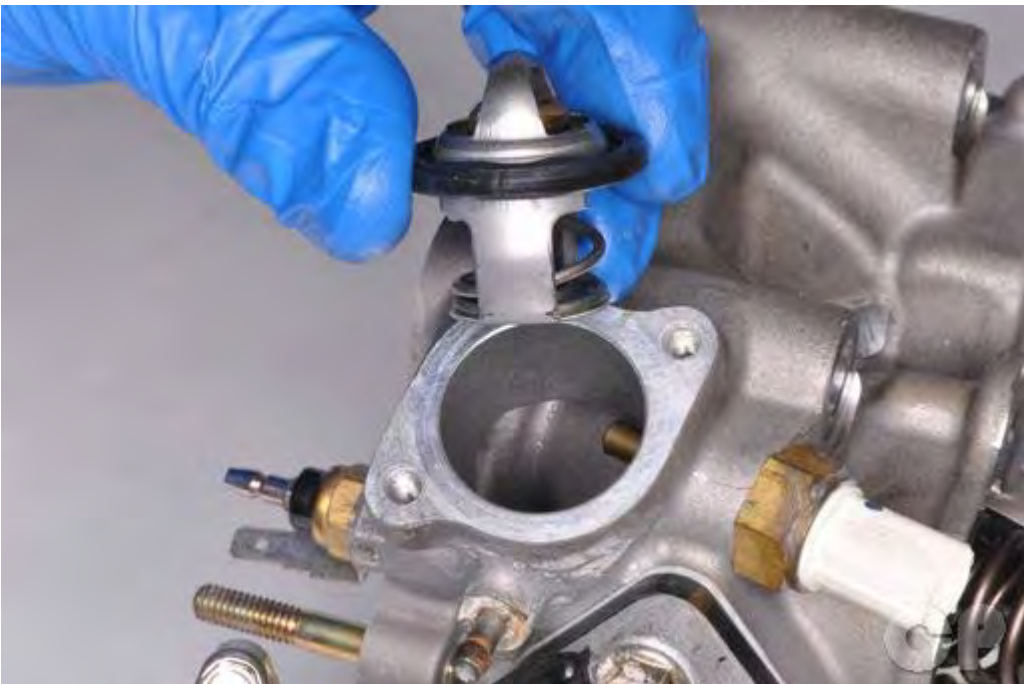
Lift out the thermostat. Remove the thermostat O-ring and discard it.
