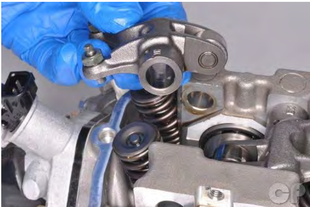
Lift out the rocker arms as the shafts are removed.
