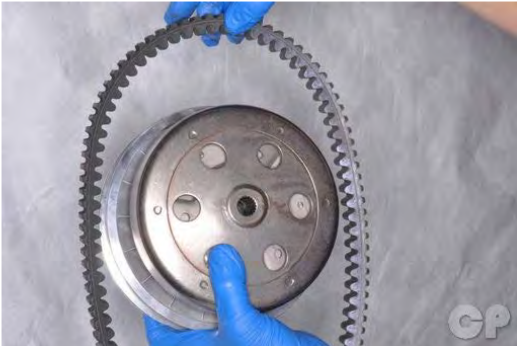
Remove the belt from the driven pulley.
