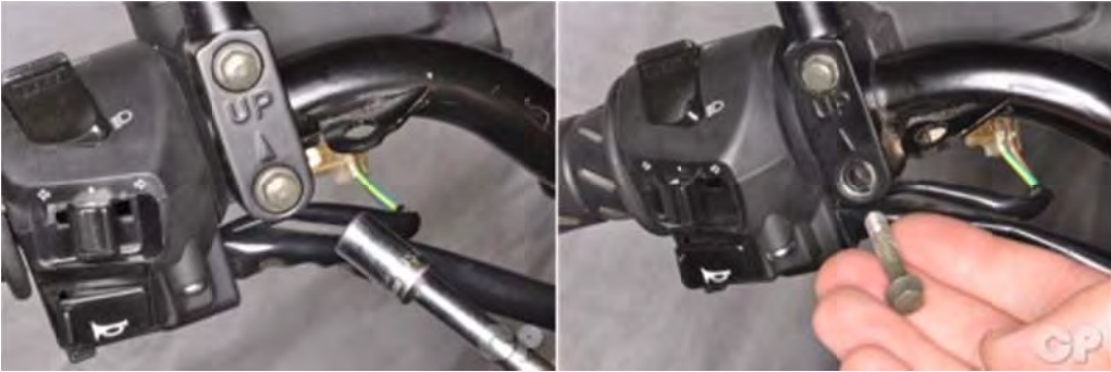
Remove the two master cylinder mounting bolts with an 8 mm socket.
