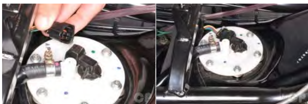
Plug in the fuel pump connector.
