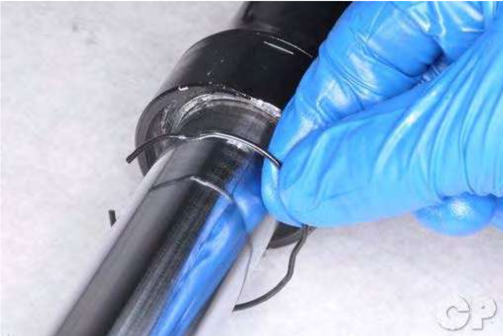
Insert the stopper ring into its groove.
