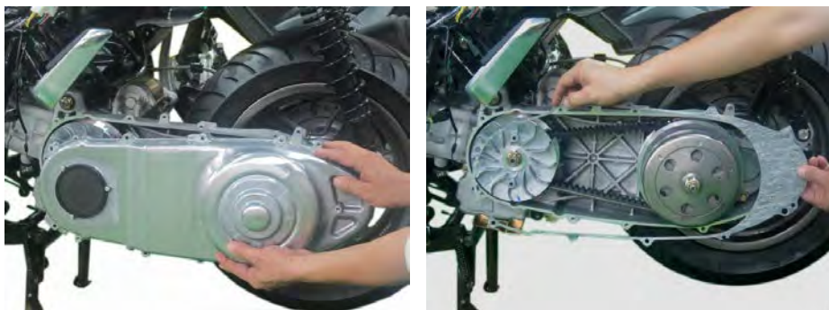
Remove the belt case cover and gasket.
