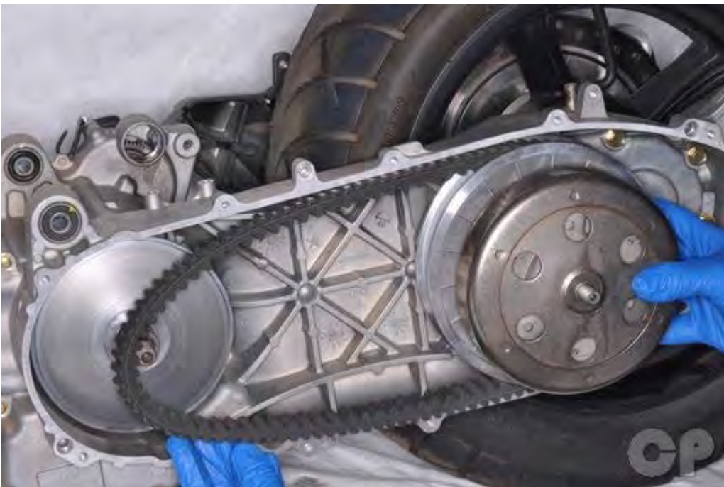
Slide the driven pulley off of the shaft.
