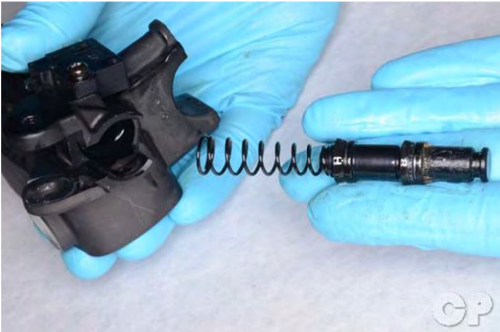
Remove the piston, spring and cups.
