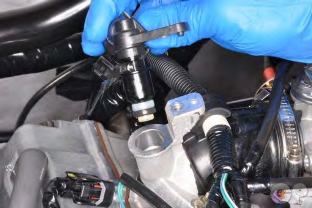
Fit the injector into the intake pipe as shown.
