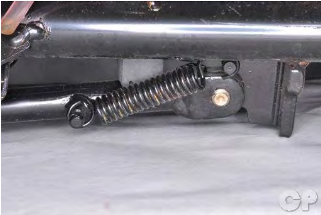
Install the side stand spring with a spring puller.
