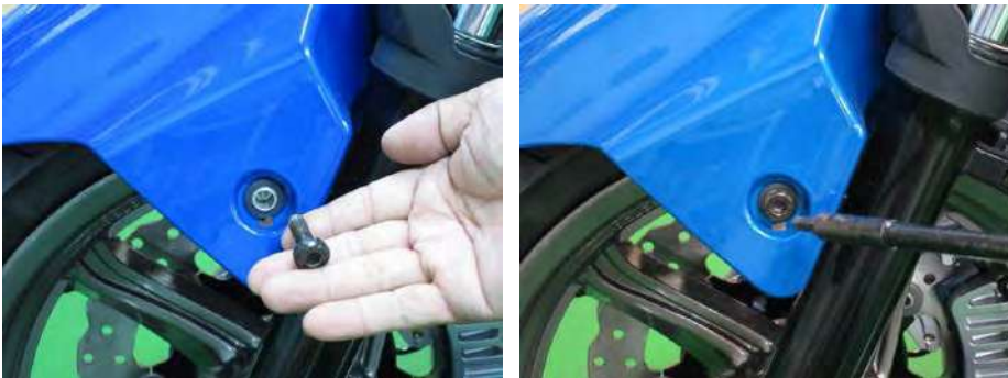
Install the left forward front fender bolt with a 6 mm Allen.
