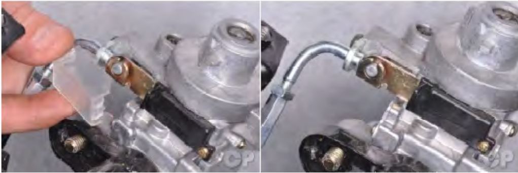
Remove the seat latch cable cover.
