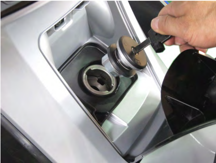
Remove the fuel cap with the key.
