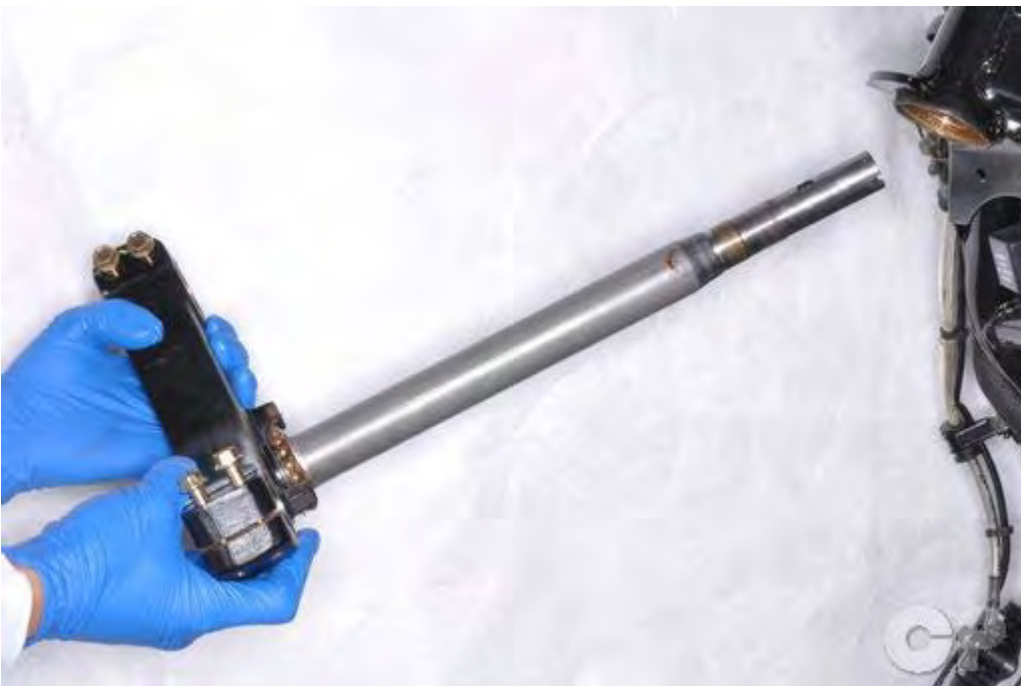
Guide the steering stem into the steering head of the frame.
