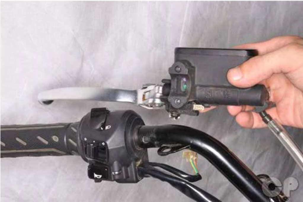
Remove the master cylinder.
