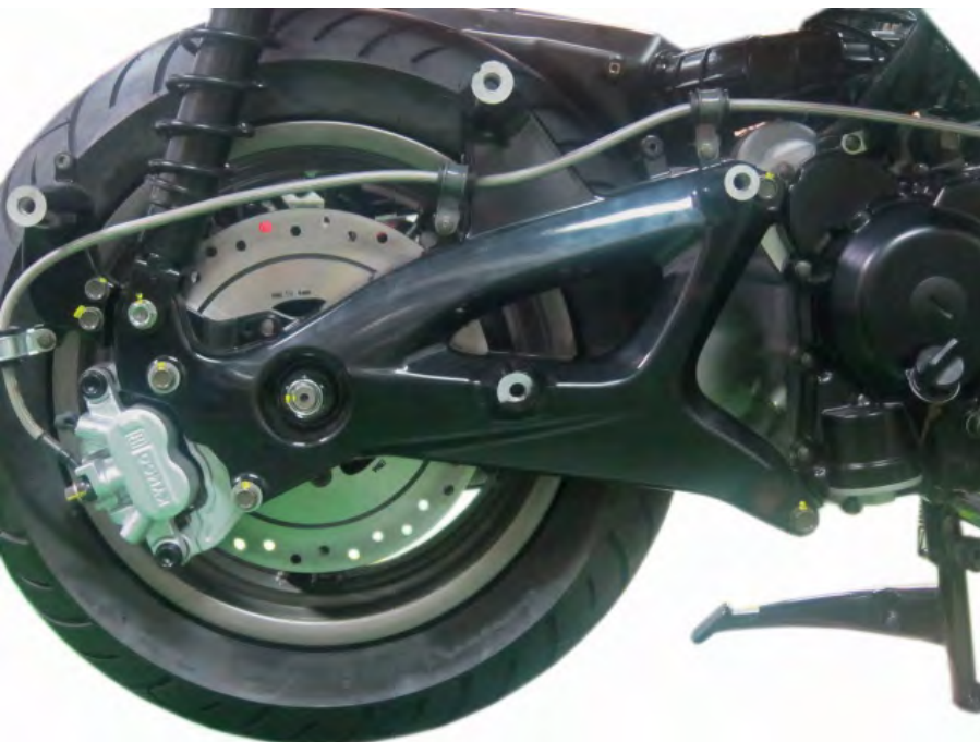
Fit the rear fork into place.
