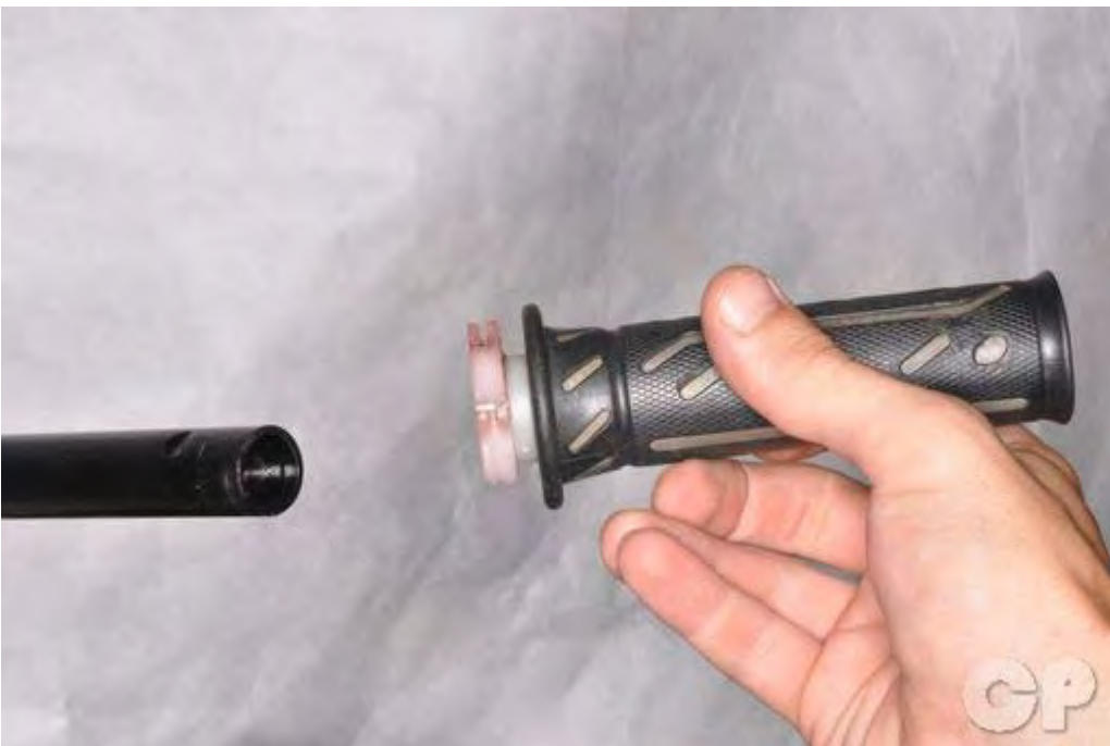
Slide off the throttle grip.
