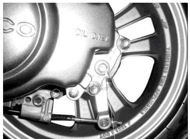
Oil Check Bolt
