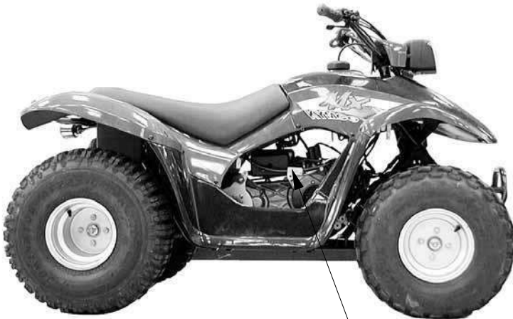
Location of Frame Serial Number
