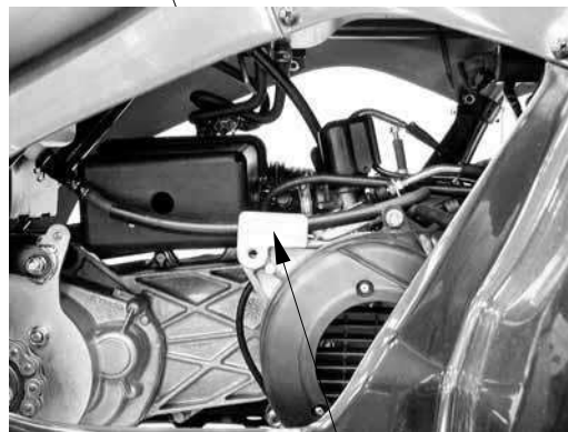
Location of Engine Serial Number
