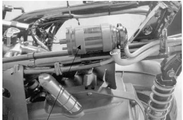
Charcoal Canister/ Purge Control Valve
